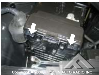
To open open the IPDM IR press on the tabs.
